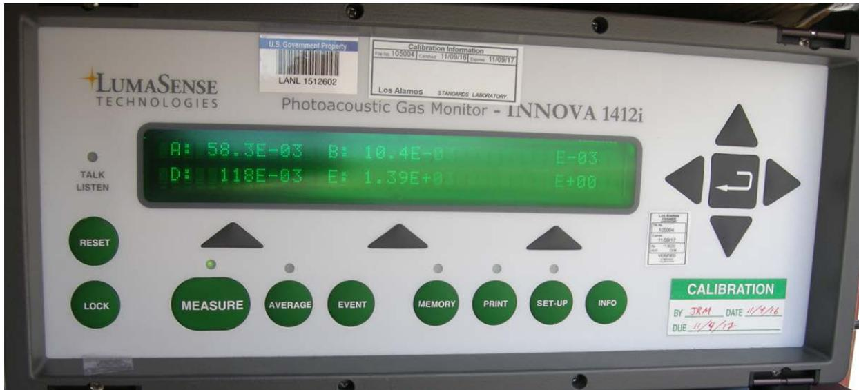
Figure 3.1-1 Innova 1412i Photoacoustic Gas Monitor, installed in the field at MDA L, April 2017.
