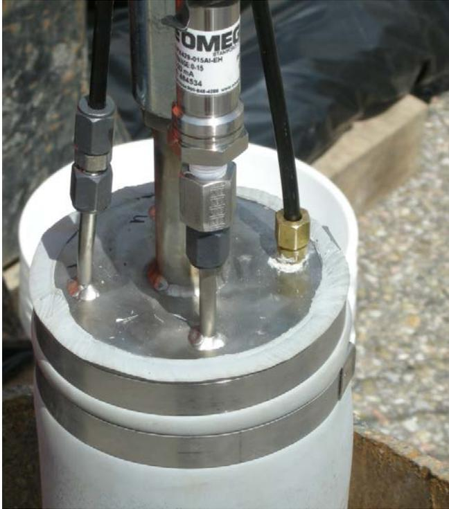
**Figure 1.2-4 Top of the permanent packer showing the OMEGA pressure transducer, one sample line and the nitrogen inflation line.**
