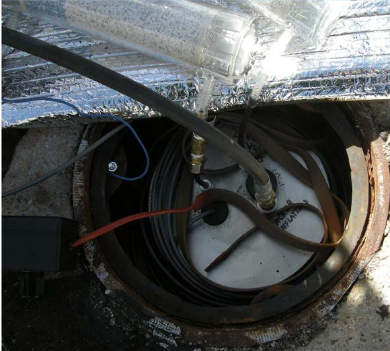
**Figure 3.2-3 Wellhead with sampling lines connected to desiccant**
