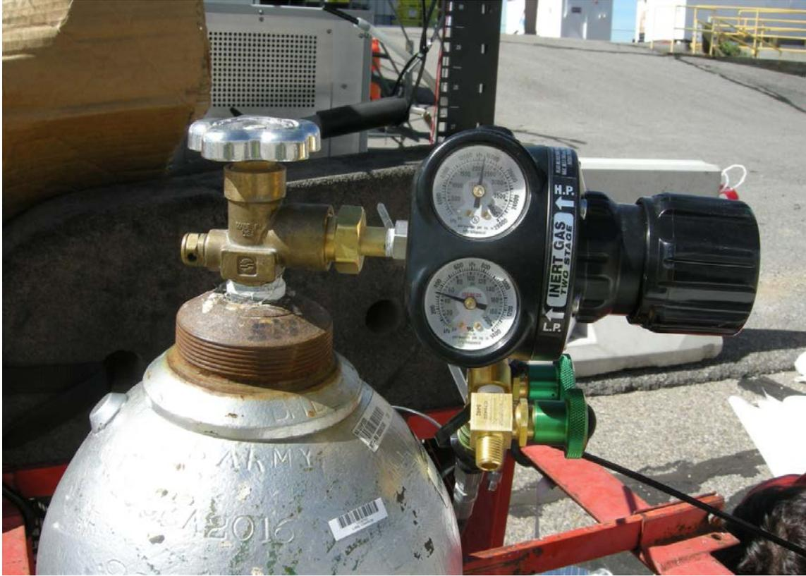
Figure 1.2-2 Nitrogen supply including pressure reduction valve.
