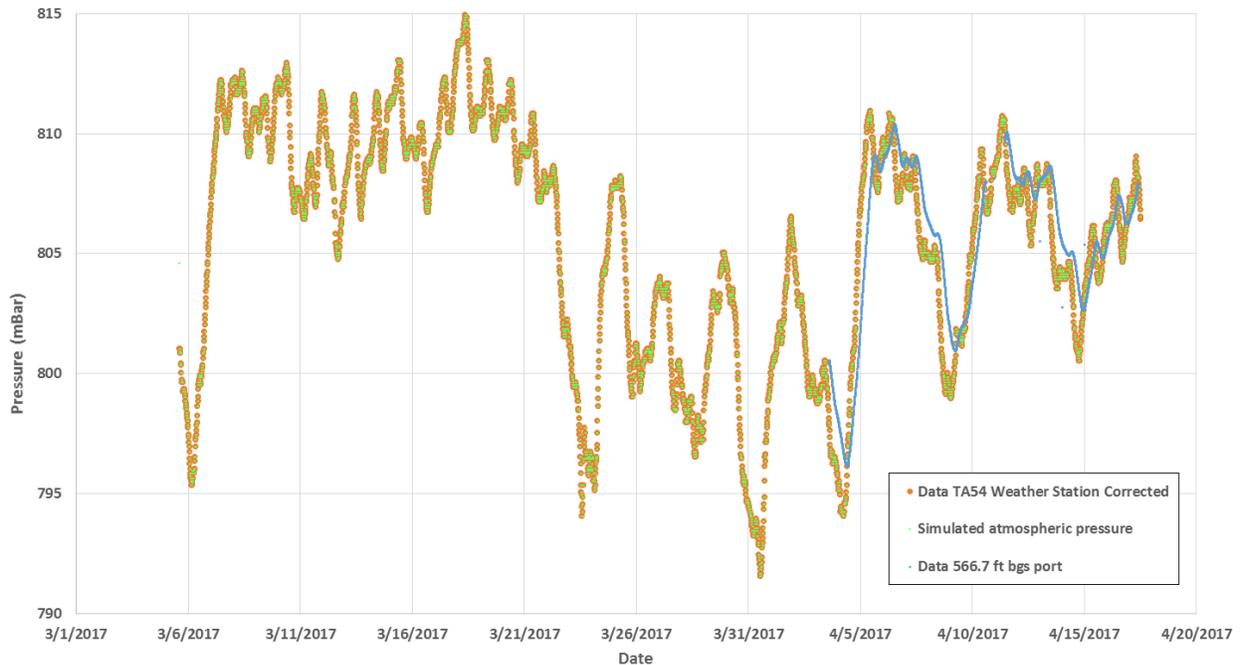
**Figure 6.3-1 Measured atmospheric pressure, March 5 – April 17 at TA-54, simulated atmospheric pressure boundary, and measured downhole pressure beneath the packer in borehole 54-24399 at 566.7 ft bgs.**
