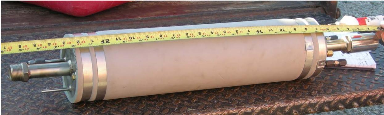
**Figure 1.2-1 New permanent packer installed in borehole 54-24399 in August 2017.**
