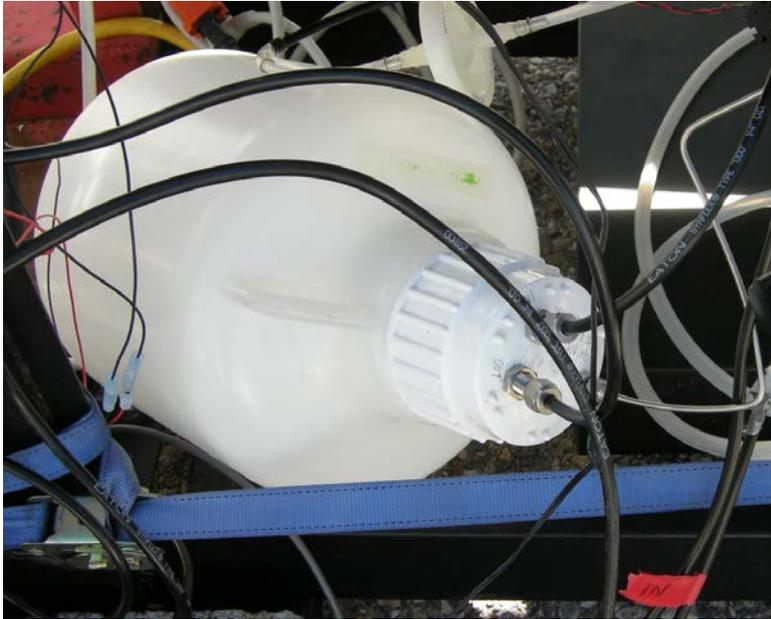
**Figure 3.2-1 10-L Carboy used as a gas reservoir to ensure continuous INNOVA operation.**
